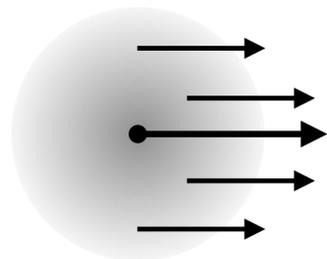
**Much later than  $t_0$ :** moving charge, with boosted Coulomb field.
